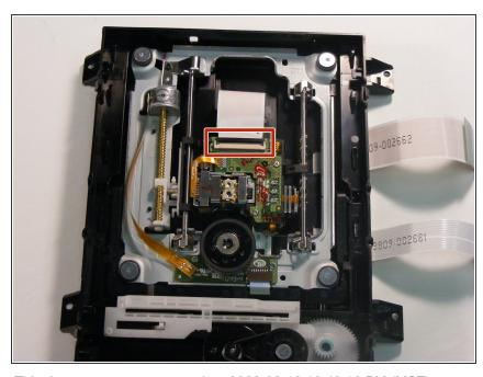
Unhook the wire from the drive lens by flipping the black piece up and pulling the wire out, at the area marked.
