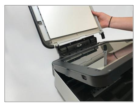
• The first thing you do is take off the top cover of the printer. After opening the snap fits, the top cover can be slid off easily.
