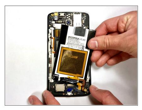
Remove the disconnected battery from the phone.
