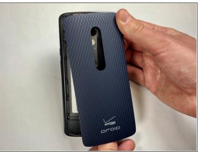
Wedge your thumb into the indent located on the bottom left corner of the back cover and pull up to remove the back cover.
