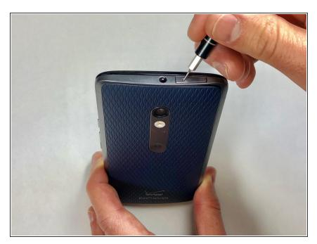
Insert a small pointed object into the hole on the sim card tray to eject the tray from the phone.
