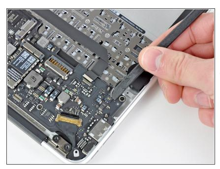
• Use the flat end of a spudger to pry the right speaker cable connector up and out of its socket on the logic board.
