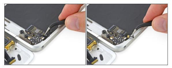
• Disconnect the microphone assembly ribbon cable by pulling it straight out of its connector.
