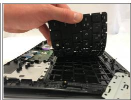
Locate the damaged keyboard and lift up with the prying tool to remove.
