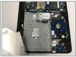
Locate the CD Compartment as shown and gently slide it out.
