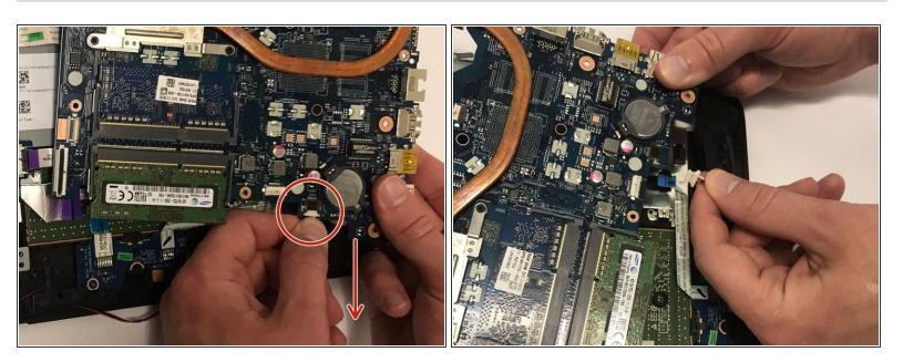
Pull out the white cable (contains red and white cable attached to a black support) with wires from its port.
