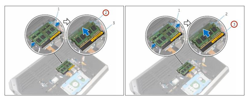
Slide and remove the memory module from the memory-module slot.
