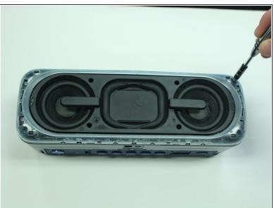
Once you have removed the outer blue casing, four T-8 screws (15 mm long) will be revealed on each corner. After removing these screws, simply pull the top part of the speaker way from the body to get the the inner part of the speaker.
