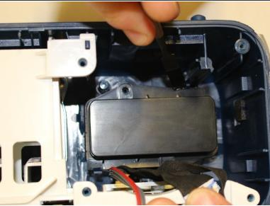
After removing the screws, pry the black cover from the base of the speaker on both sides using a metal spudger.
