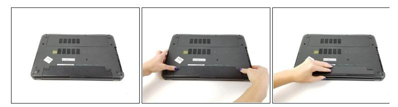
Remove the battery to avoid electrical discharge while working with this system.
