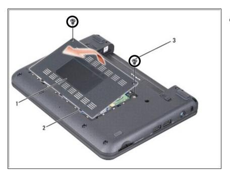
• Remove the two screws on the module cover.
