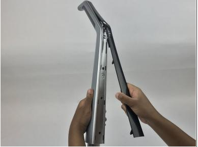
• Use a plastic opening tool to carefully pry the black cover off of the handle.
