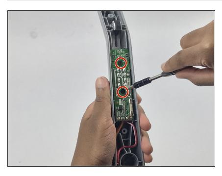
Remove two 8mm Phillips #1 screws from the motherboard.
