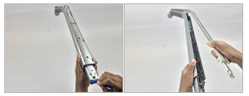
Remove the silver plastic cover using the plastic opening tool.
