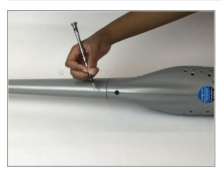
Remove the single 15mm Phillips #1 screw from the handle.
