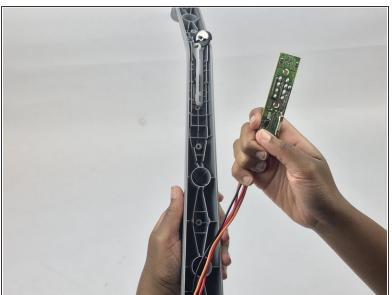
Carefully pull the motherboard out with its attached wires.
