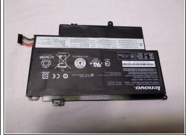
Carefully pull the connector out from underneath the logic board to remove the battery.
