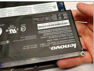
Carefully lift the battery. There is a small bit of adhesive underneath the green.
