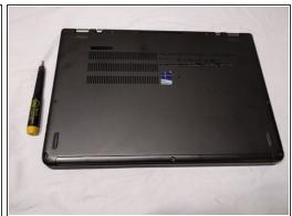
Remove the ten Phillips screws using a Phillips 00 screwdriver
