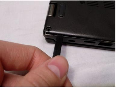
• Pry up the case carefully using a spudger.
