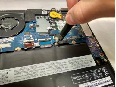
Remove the one and only Phillips screw with a Phillips 0 screwdriver.
