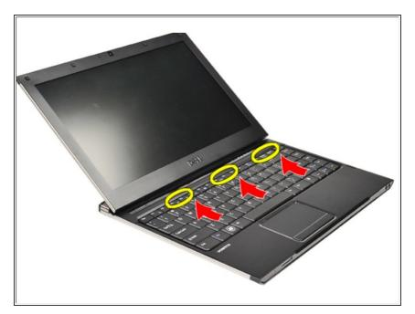
• Starting on the right side of the system, use a plastic scribe to pry up the LED cover from the computer.
