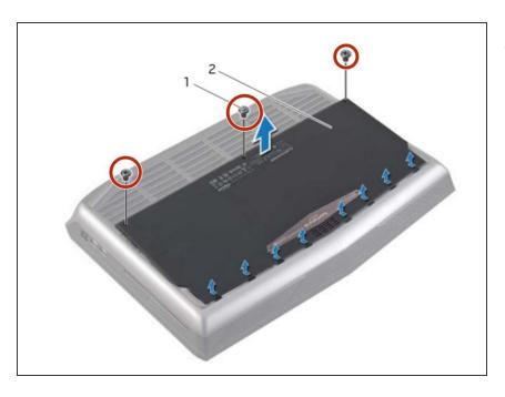
Use a Phillips screwdriver to remove the three screws securing the base cover.
