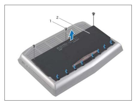
Slide the base cover towards the rear of the computer and lift it off the computer base.
