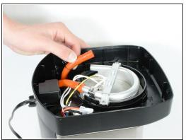
Gently pull on the loose hose to remove it from the heating element.
