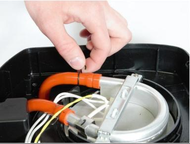
Gently squeeze the hose clamps together and begin moving the metal clamp away from the heating element.
