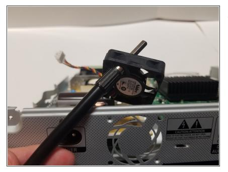
The fan is now free from its screws and wire and can be freely lifted out of the casing.
