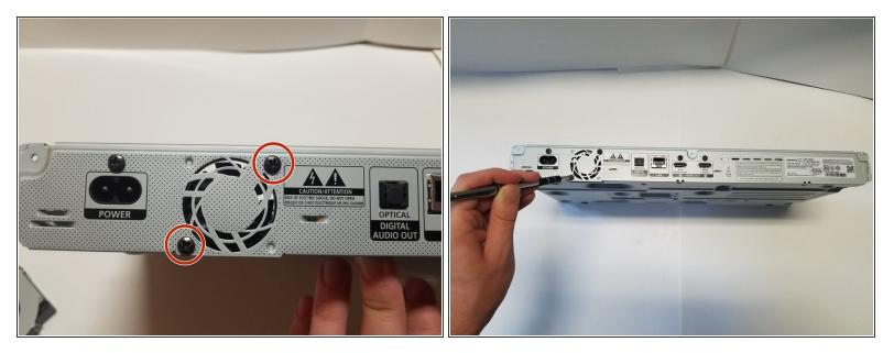
• Using a #1 phillips head screwdriver, remove the two 8.1 mm screws in the corners of the fan.
