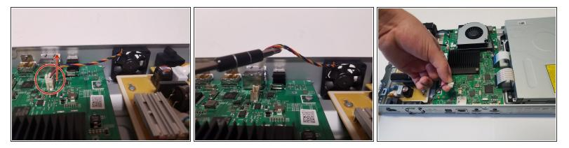
• Use your fingers to pinch the white tip of the multicolored wire connecting the fan to the motherboard. While pinching, gently pull up to remove the wires from the motherboard.
