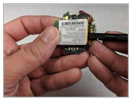
The battery is glued to the motherboard and will need pried off using the nylon spudger.
