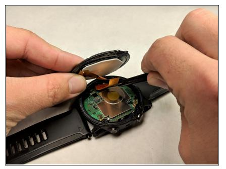
Proceed to disconnect the ribbon from the motherboard using tweezers.
