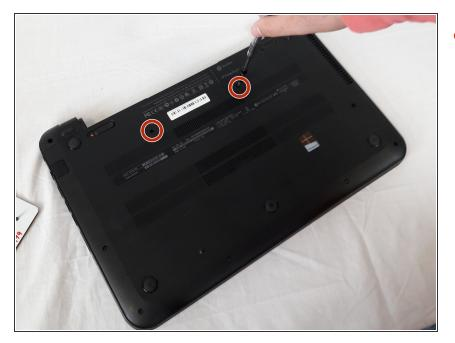
Remove the two 6.5mm Phillips #1 keyboard screws from bottom of laptop.
