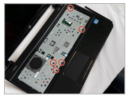
Remove the five 5.5mm Phillips #1 screws from the case
