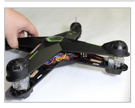
Separate the upper and lower housing units by lightly pulling the two housing units apart. To reassemble your device, follow these instructions in reverse order.
