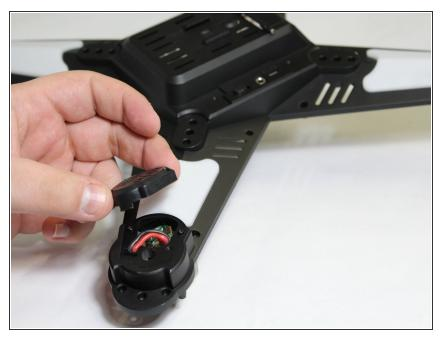
• Remove the motor cover by lightly pulling it away from the drone.
