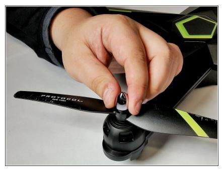
• Remove the chrome shaft cover by lightly pulling it away from the drone.
