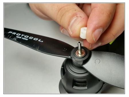
Remove the propeller stop from shaft by lightly pulling it away from the drone.
