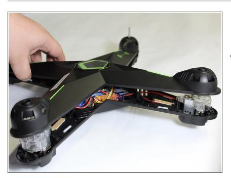
Separate the upper and lower housing units by lightly pulling the two housing units apart.
