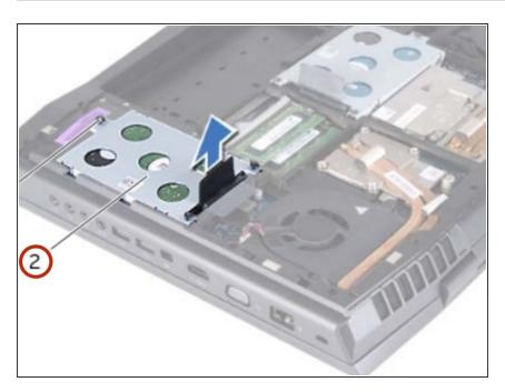
Lift the hard-drive assembly out of the computer base.
