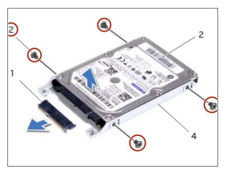
Remove the screws that secure the hard drive to the hard-drive bracket.
