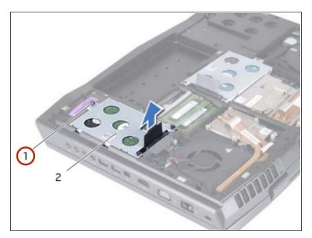
Tighten the captive screws that secure the hard-drive assembly to the computer base.
