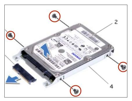
Replace the screws that secure the hard drive to the hard-drive bracket.
