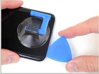
Slide your opening pick along the lower edge of the display to separate the adhesive underneath.
