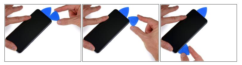
Use your opening pick to separate the adhesive under the left side of the display.
