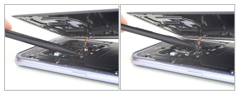
• Use the point of a spudger to pry up and disconnect the fingerprint sensor flex cable.
