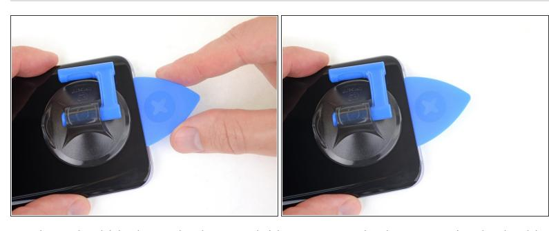
• Leave the pick in place and grab a second pick as you proceed to the next step. Leaving the pick inserted can help prevent the glue you just separated from re-adhering.
