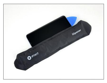
Reheat the iOpener and apply heat to the left edge of the display for at least two minutes.
