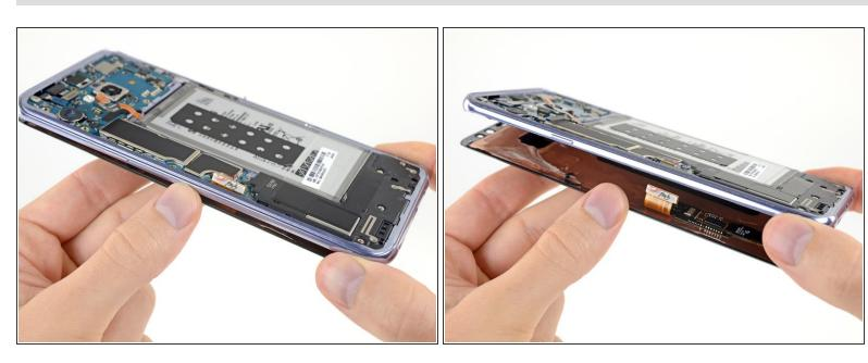
Route the display's flex cable through its hole in the frame in order to fully separate the right edge of the display.
