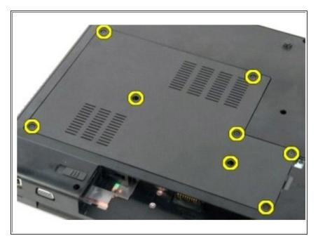
Remove the eight screws from the access panel.
