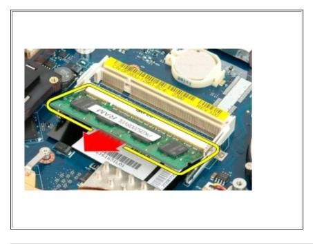
Slide the memory module out of the socket.
