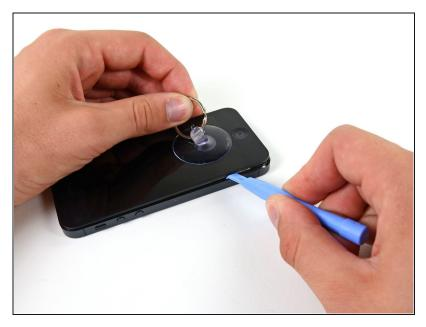
• Continue to pry up around the sides of the front panel assembly, detaching the clips along the left and right side.
