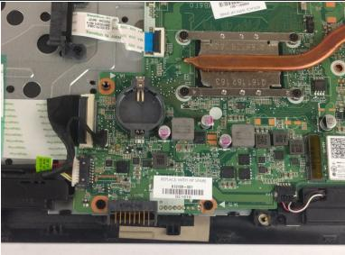
Lift up until battery pops out, remove battery
