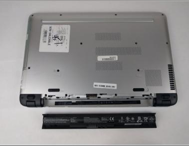
Grabbing the top edge of the battery, rotate it toward you and then lift upward to relieve the battery from its slot.
