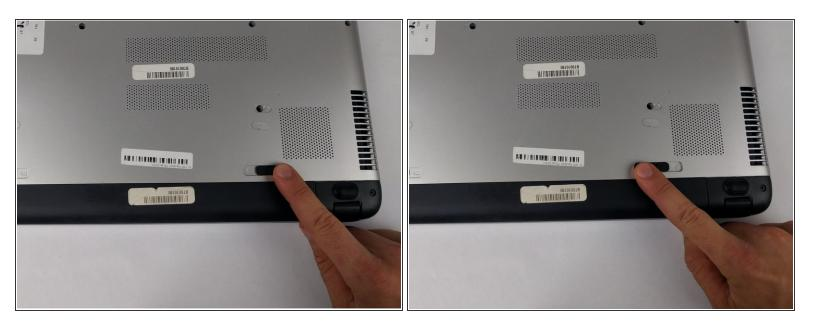
Slide the battery lock tab toward the center of the battery to the unlock position.
