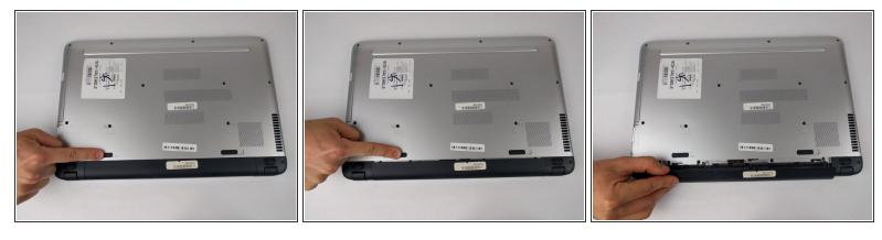
Slide the battery release switch to the right until the battery pops out.
