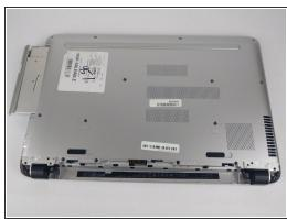
Remove all 16 of the 3.5 mm screws with a PH1 screwdriver and pry/slide the CD drive out of laptop.
