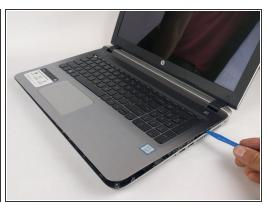
Using a plastic opening tool, begin to pry edge of case away from the laptop. Work around the edges until all sides, except back, are open.
