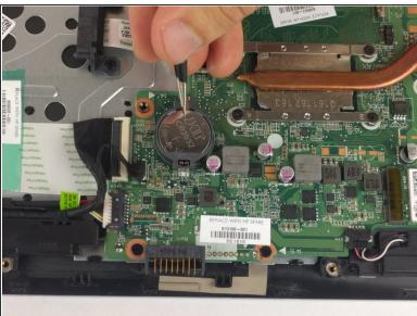
Use long nose tweezers to reach under battery and lift up.
