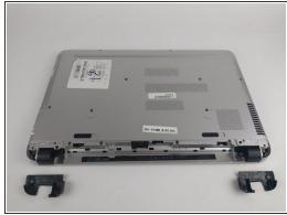
With the battery removed, remove both black plastic covers with a plastic opening tool. Unscrew both 7.5 mm screws from the tabs, using a PH1 screw driver. Using a plastic opening tool, pry off both covers.
