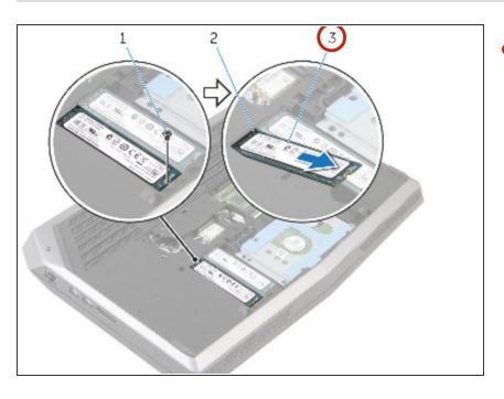
Slide the solid-state drive into the solid-state drive slot.
