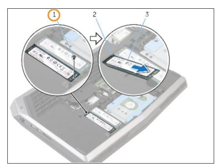
Align the screw hole on the solidstate drive with the screw hole on the computer base.
