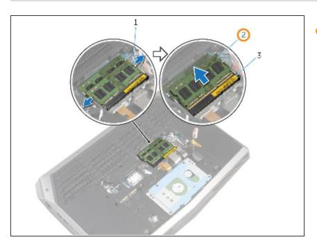
Slide and remove the memory module from any memory-module slots that you would like to repopulate.
