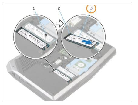
Slide and remove the solid-state drive from the solid-state drive slot.
