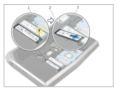
Replace the screw that secures the solid-state drive to the computer base.
