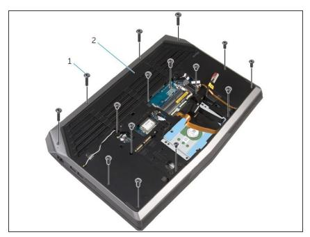
Remove all 15 screws which hold down the computer base. Two screws are located near the RAM slot, while the others are situated mostly around the outside of the computer.
