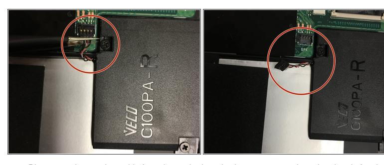
Disconnect the speaker cable from the motherboard using tweezers or the pointed end of a plastic spudger.
