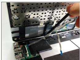
Disconnect the touchpad cable and the keyboard cable on the palm rest assembly from the motherboard using the pointed end of a plastic spudger.
