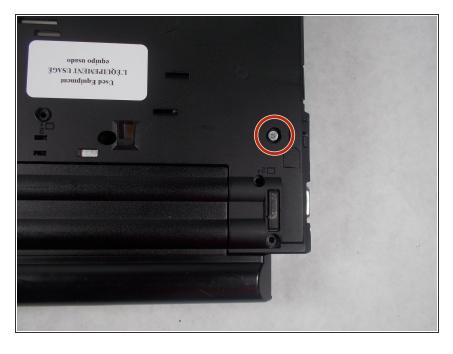
Remove the screw to be able to use the CD drive unlock switch
