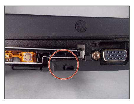
Locate the switch on the right side of the CD Drive.
