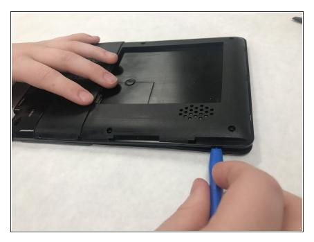
• Pry open the casing with a plastic opening tool .
