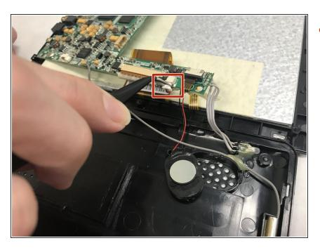
• Pry the speaker clip from the motherboard using tweezers.
