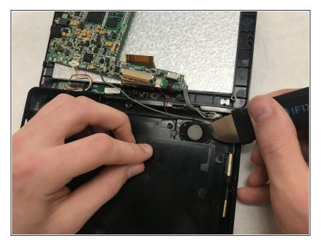
• Pry the speaker out of retainer clip with iFixit pry tool.
