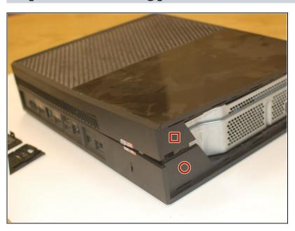
• To disconnect the top it has a series of clips to unhook the first is tricky, you want to start by pushing the piece with the red square back toward the device while simultaneously pulling the part with the circle toward you, lifting it in an upward direction to separate them.
