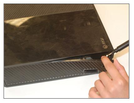
First start by locating the side of the console with the sync button or USB slot. Then carefully pry the side panel from the Xbox until it is completely separated.
