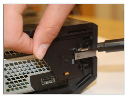
After removing the panel behind the silver sync button remove its brace by using a screw driver to slide it out toward the backside of the Xbox.
