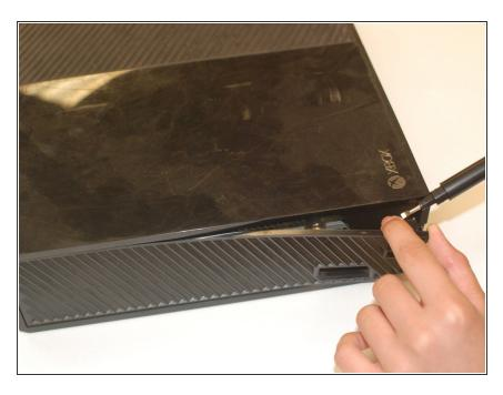
First start by locating the side of the console with the sync button or USB slot. Then carefully pry the side
