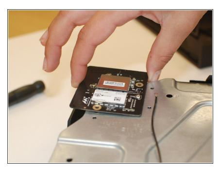
Now everything is disconnected from holding the card down you want to carefully pull the card straight up from the console until separated.
