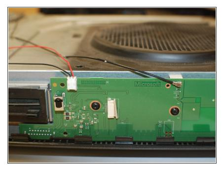
Now make your way back to the front and connect the front wires the white one should slide down and clip into place and the black will snap down.
