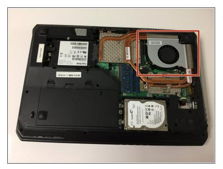
Locate the CPU Fan inside the computer. It is outlined in red.
