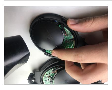
Use a heat gun to carefully loosen the glue on the speaker cover.
