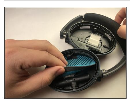
Next, remove the soft lining behind the cushion. This is held on with adhesive and is easily removed by hand.
