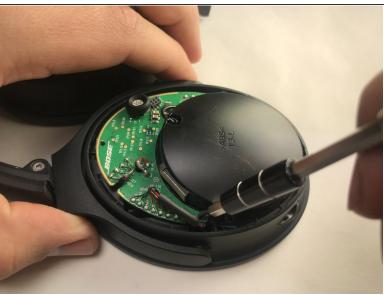
Once the inside of the headphone is exposed, use screw driver (PH00) to remove the two 4mm screws on the black speaker cover.
