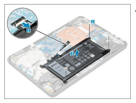
Connect the battery cable to the connector on the battery.
