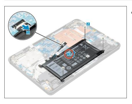
Insert the **NEW** battery into the slot on the computer.
