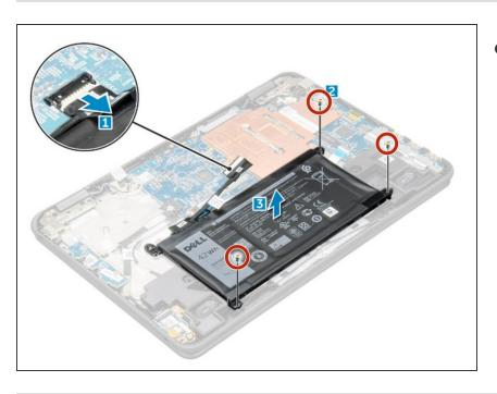
Replace the M2.0x3.0 screws to secure the battery to the computer.
