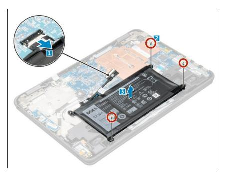
Remove the M2.0x3.0 screws that secure the battery to the computer.
