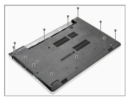
Flip the computer and remove the screws (8 screws - M2.5L8; 3 screws - M2L2; 2 screws- M2L2) that secure the base cover to the computer.
