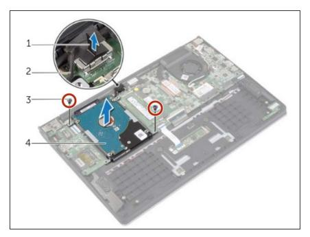
Replace the screws that secure the hard-drive assembly to the palm-rest assembly.
