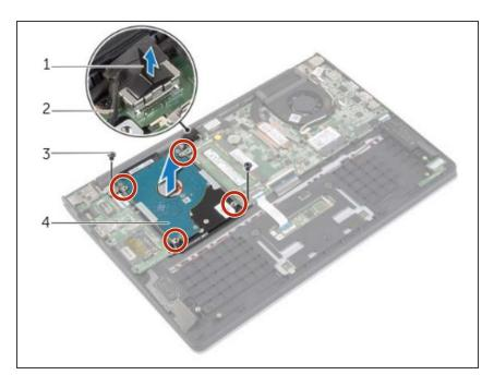
Align the screw holes on the harddrive assembly with the screw holes on the palm-rest assembly.
