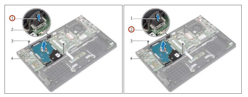
• Using the pull-tab, disconnect the hard drive cable from the system board.
