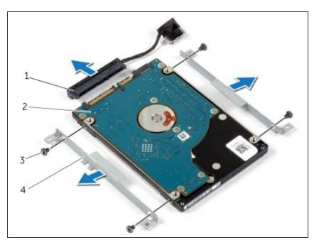
Align the screw holes on the NEW hard drive with the screw holes on the hard-drive bracket.
