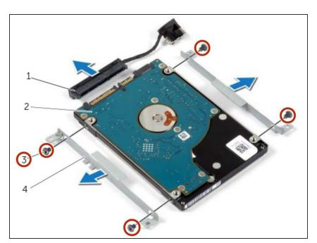
• Remove the screws that secure the hard-drive brackets to the hard drive.
