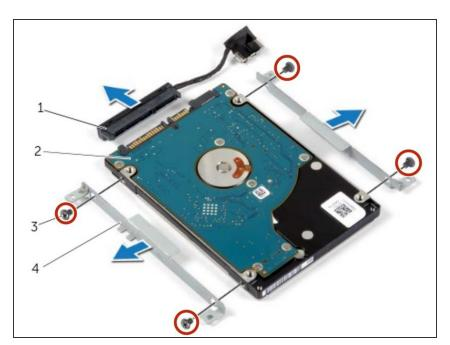
Replace the screws that secure the hard-drive brackets to the hard drive.
