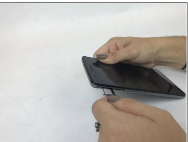
Use the Sim card ejection tool to remove both the sim card trays.
