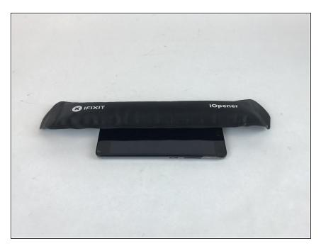
To prepare the iOpener insert it in the microwave for 30 seconds and apply it on the side edges of the phone so that the glue underneath will soften.
