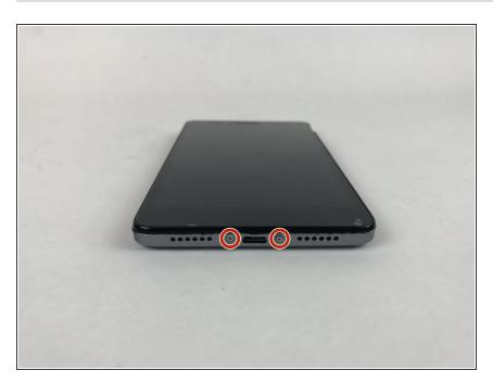
Remove the two 1.17mm Torx T3 screws from the bottom of the phone.
