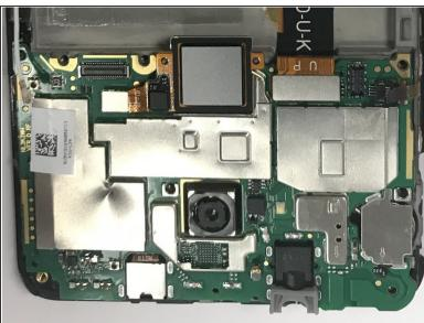
Remove the five 1.5mm Phillips #000 screws from the motherboard.
