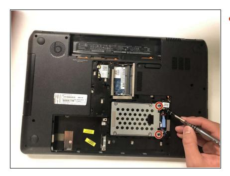
Remove the two Phillips #00 screws holding in the hard drive.
