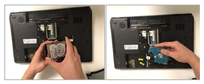
• Slide the casing off of the hard drive.
