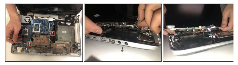
• Use the flat end of a spudger to disconnect all wires connected to the motherboard.
