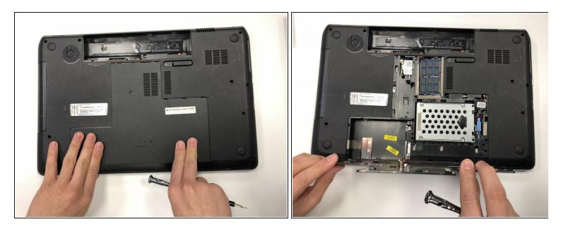
• Remove service hatch by sliding away from the computer and lifting up.
