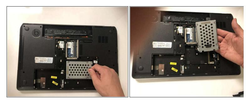
• Grab the black tab on the hard drive and pull left and then upwards to remove.
