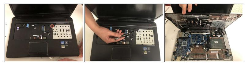
Use Phillips #00 to unscrew the screw and take off the front panel.
