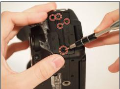
• Using a metal spudger, pry the rubber grip off of the casing on the left side of the camera.
