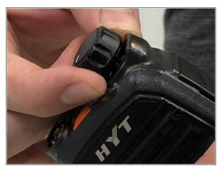
• Remove the volume knob by firmly lifting up on both sides of it.
