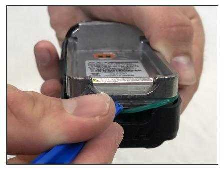
• Using a plastic opening tool, pry in between the plastic case and metal circuit board to remove the board.
