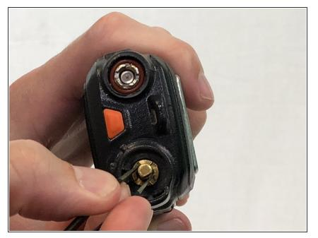
Remove the brass washer from the base of the antenna slot by turning it counterclockwise with a set of tweezers.
