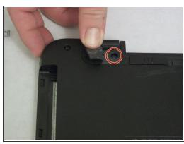
With the laptop upside down, remove the battery by hand and the twelve 7.0 mm screws that are holding the back case to the front. Use a JIS #0 screwdriver to remove the screws.
