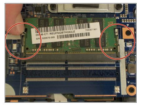
Using your finger, pry the metal clip from both sides of the RAM module and the module will "pop" up.
