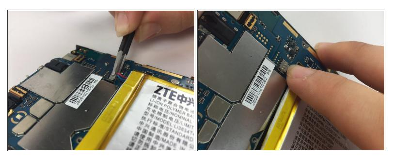
Disconnect the battery from the motherboard.
