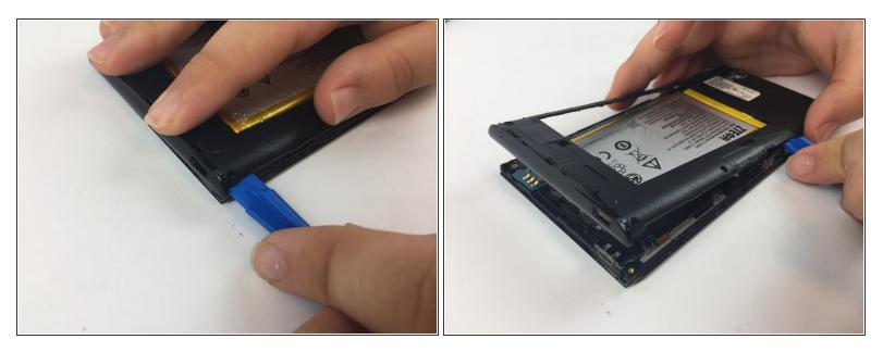
• Remove the mid frame with the plastic opening tool.
