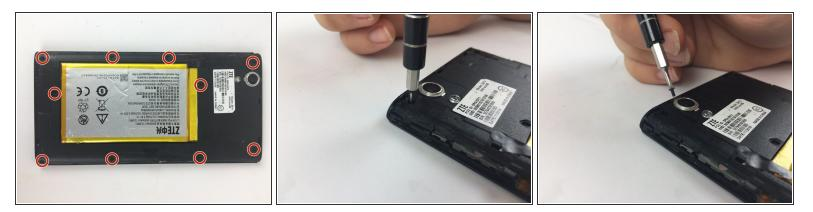
• Remove the ten 1.2mm screws with a Phillips #000 screwdriver.
