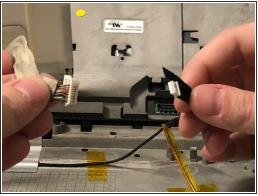
• Disconnect the display connectors by removing them from the grooves and unplugging them.
