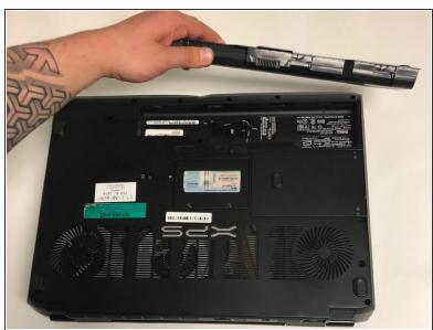
Lift and remove the battery.
