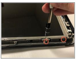
Remove 12 M2x3mm screws along the edge of the screen frame with a PH0 screwdriver.
