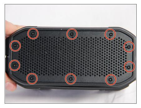
To remove the front speaker screen, unscrew the 10 Hex 3mm bit type, 9mm long screws surrounding the screen.
