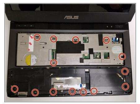
Remove the fourteen Phillips #0 screws.
