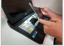
Insert a spudger, or plastic opening tool, into these five slots and pry upwards to pop up the keyboard.
