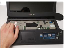
Insert your screwdriver into the locking mechanism and slide it to the left. This will unlock the hand rest and allow you to pull it free.
