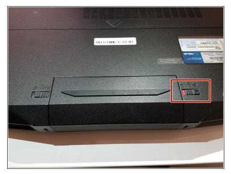
Unlock the battery by pushing the switch to the right.
