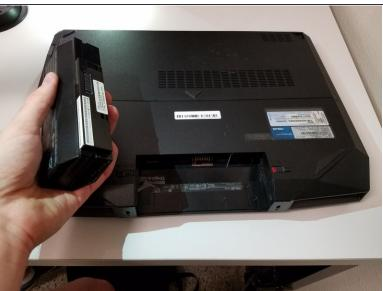
Push and hold the left switch, then pull the battery out.
