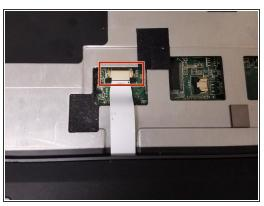
• Disconnect the keyboard ribbon cables from the motherboard.
