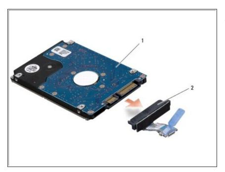
Pull the interposer to disconnect it from the hard drive.
