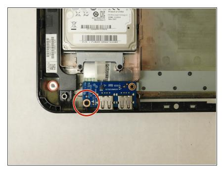
Remove the single screw holding the USB ports and chip into the computer.
