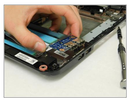
Remove the chip by gently pulling it up and then away from the edge of the case.
