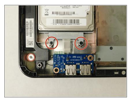
Remove the 2 black screws holding the hard drive to the computer frame.
