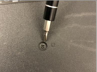
Using a Phillips #1 screwdriver, remove the small screw next to the disc engraving shown in the picture.
