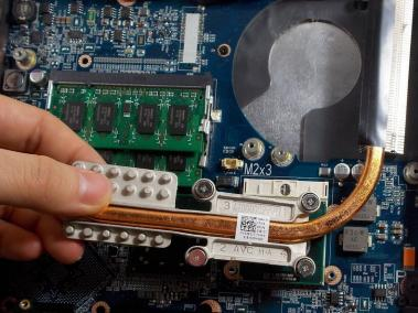
Lift up on the heatsink to remove it from the laptop.
