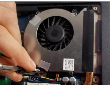
Remove the two 3mm screws located around the edge of the fan with a Philips #1 screw driver.
