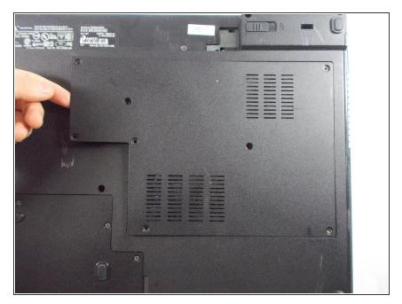
Lift back cover from the groove on the left side of the cover next to the symbol.
