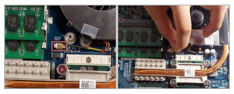
Unclip the power supply by pulling the cable directly up and out of the socket.
