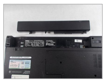
Remove the battery from the slot.
