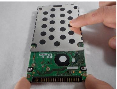
Holding the hard drive in place with the connection facing towards your body, put a finger on the cover and slide it away from your body to reveal the hard drive.
